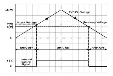
Output offset detection protection circuit
