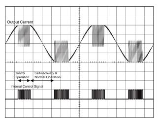
\* The over-current protection circuit functions only to avoid the abnormal state, such as output short-circuit, etc., temporarily, and does not guarantee to offer the protection to prevent damage to IC.
